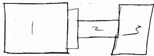
$$\begin{array}{c} 2.00 \pm .01 \\ | \quad \quad \quad | \quad \quad \quad | \\ 1.00 \pm .02 \quad 1.00 \pm .05 \\ | \quad \quad \quad | \\ 4.00 \pm .08 \rightarrow \end{array}$$
